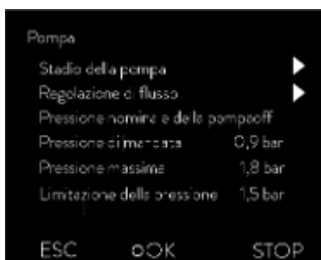
Fig. 44: Menu pompa Integral XT FC
